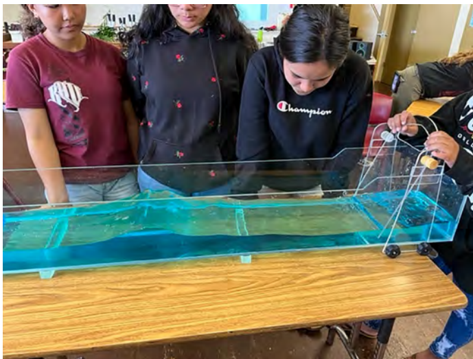
Figure 4. Creating a standing wave in a wave tank to understand a natural phenomenon in the ocean.
