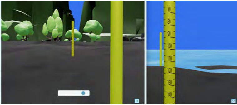
Figure 3. A simple method of measuring beach profiles on the ground is enacted using a simulation. Students work in teams with one student viewing seaward and lining up their measuring rod with another student whose view is facing landward.
