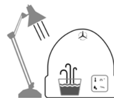
Figure 1. A heat lamp outside a microbiome with temperature and humidity sensors inside the enclosure.
