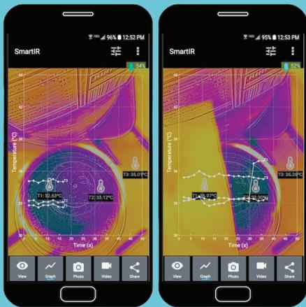
**Figure 1.** SmartIR app running on a mobile phone records thermal imaging data.
