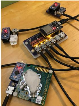
**Figure 2.** A Dataflow program created by a ninth grade biology student during the Stabilization Lab unit. The program actuates a red-blue LED lamp connected to a relay, and stores and graphs CO<sub>2</sub> and light data during the experiment. When CO<sub>2</sub> levels in the container reached above 1,000 PPM, the student's lamp turned on, initiating photosynthesis in the spinach leaves, which then caused the CO<sub>2</sub> levels to decrease.
