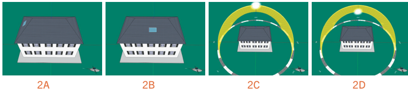
Figure 2. Screenshots of student work from Energy3D. Images A and B reflect the first practice (moving the solar panel from the eastern side of the roof to the northern), and C and D the second practice (only the heliodon on June 22 and December 22 are shown). Note: All images are looking south.
