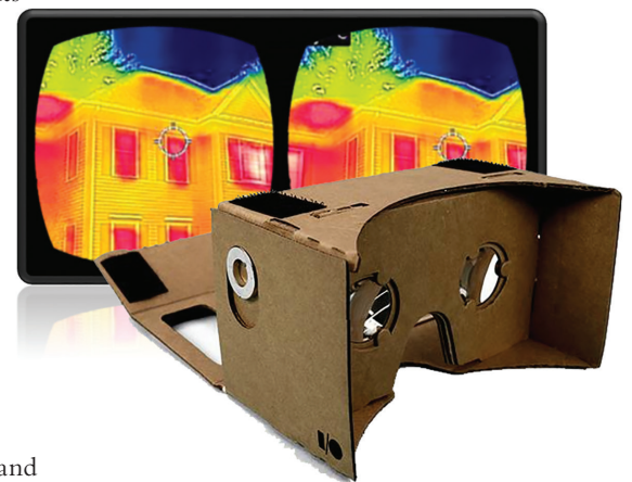
Figure 1. We imagine an immersive thermal vision. Based on the orientation and GPS sensors of a smartphone, SmartIR can create a thermogram sphere and then knit images together to render a seamless IR view. Virtual Infrared Reality can be uploaded to Google Maps so the public can experience it using a VR viewer, such as Google's Cardboard Viewer.
