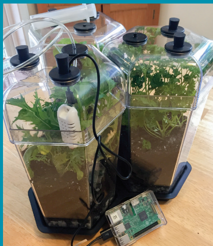
Figure 1. Growth chambers made by PASCO connect to a credit card sized Raspberry Pi computer wirelessly connecting virtual Dataflow programs with physical sensors and actuators in experiments.
